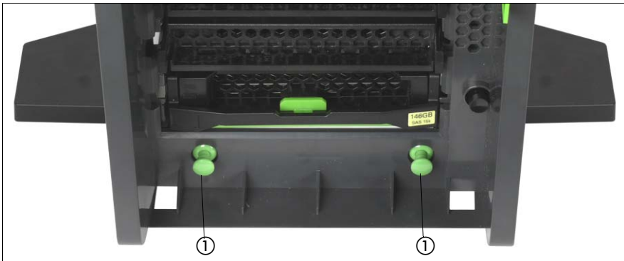
Figure 82: Locking buttons engaging
